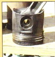
All the pistons had piston skirts and piston rings totally clean of any build-up. The rings looked like new and didn't have any wear.
