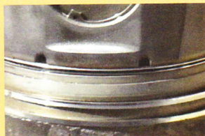
All the pistons had piston skirts and piston rings totally clean of any build-up. The rings looked like new and didn't have any wear.
