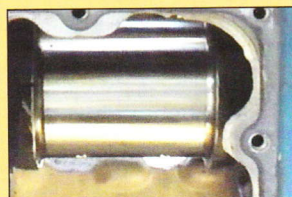
We micro-measured the crankshaft and found it to be in great condition. Totally round, no traces of wear. It didn't need any machining.
