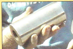
After 30,000 work-hours in operation and 100 hours in the presence of water, all the piston pins didn't have any traces of wear, looked polished like and new.
