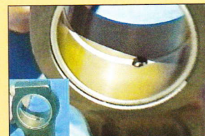
After 30,000 work-hours in operation and 100 hours in the presence of water, all the piston pin bearings didn't have any traces of wear, looked like new.
