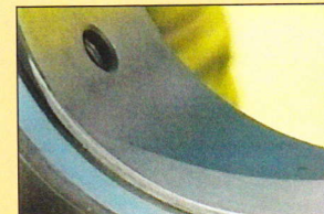
After 30,000 work-hours in operation and 100 hours in the presence of water, all the connecting-rod bearings didn't have any traces of wear, maintained their full thickness and their coating. They looked like new.
